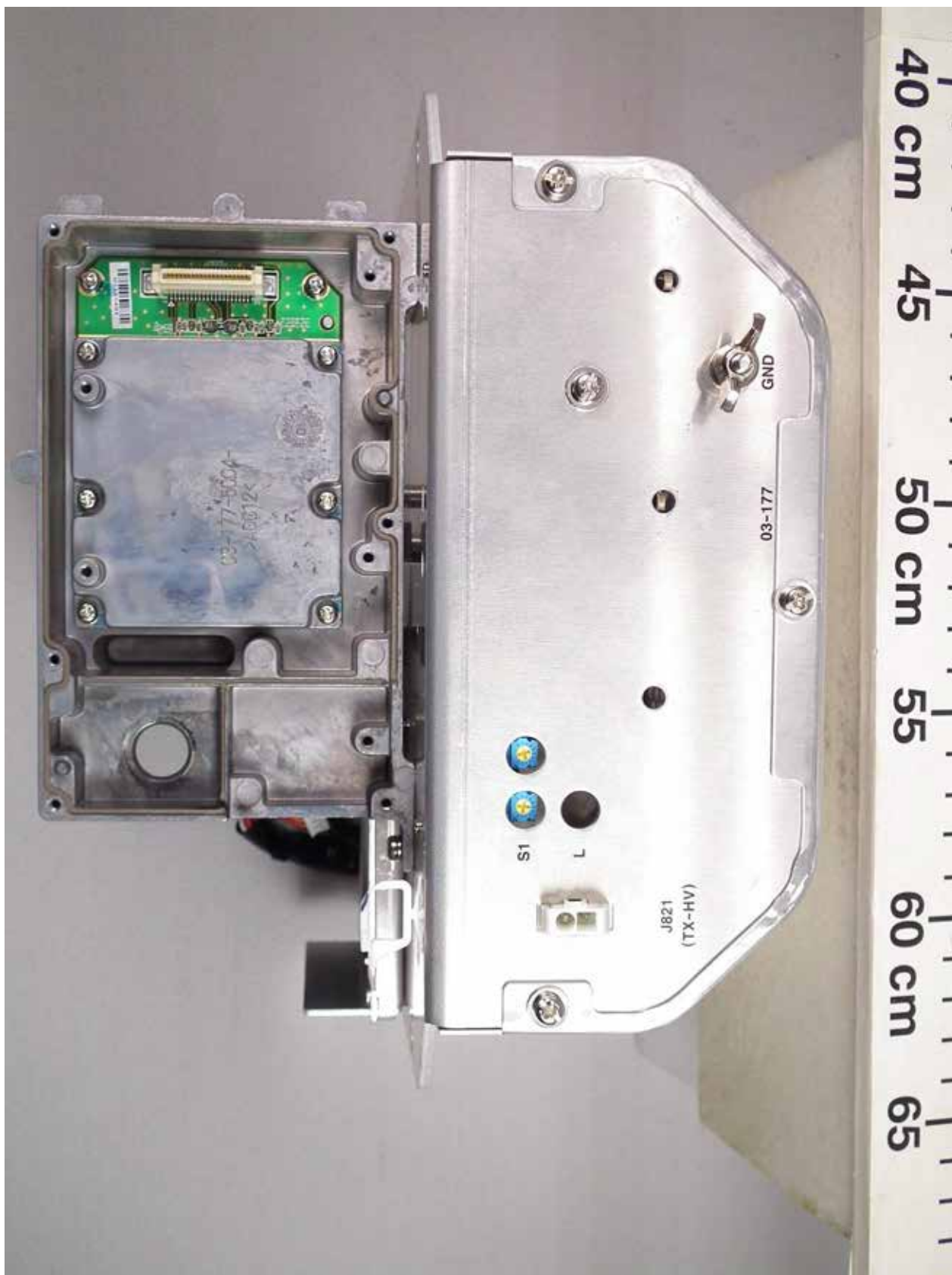
1.6 Front side view (with IF Board removed, showing MIC Board 03P9505 inside)
