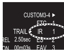
"IR" (Interference rejection) icon (at the bottom right corner on the screen)
