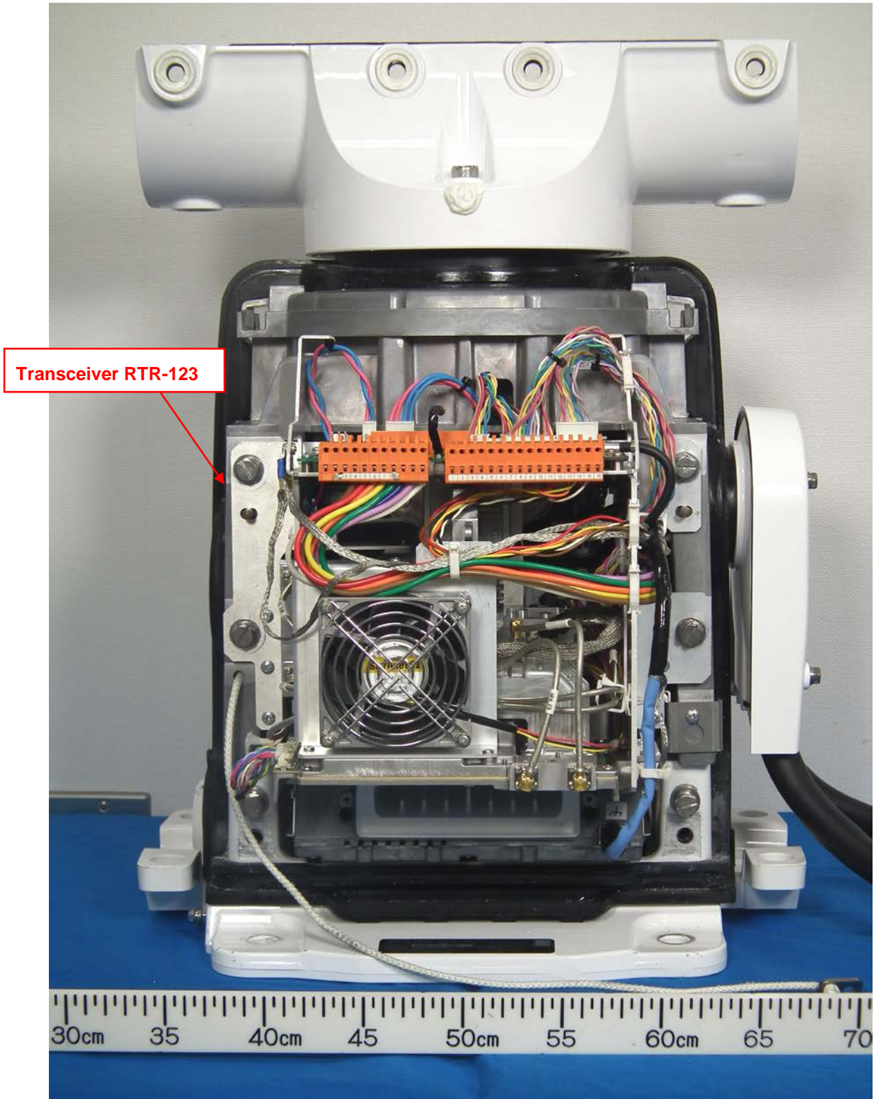
1.1.3 Rear view of RSB-128 (with the rear cover removed, showing Transceiver RTR-123)
