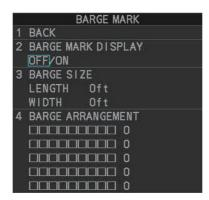
5. Select [ON] to display barge marks, [OFF] to hide barge marks, as appropriate, then press the **ENTER MARK** key.
