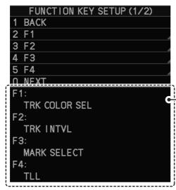
When [SINGLE] is selected as the key mode, the current setting for the function key is shown here. Function keys with [MULTI] selected as their mode are hidden.
