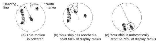
**Note:** The position of the own ship marker and bearing scale change according to reference position and off-centering.
