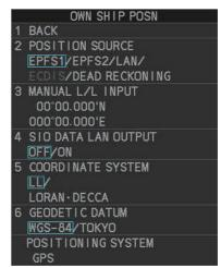
6. If [2 POSITION SOURCE] is selected at step 2, select the appropriate position source, referring to the list below, then press the **ENTER MARK** key. [2 POSITION SOURCE] uses navigational aids. Select the navigational aid to use. Available options are listed with a brief description in the table below:
