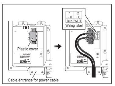
5. Remount the plastic cover and the front cover, then clamp the power cable on the sheath.
