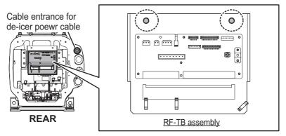
4) Wrap the supplied spiral tube around the de-icer power cable, starting from the crimp-on lugs. Set a locking wire saddle (supplied) at location (5) shown in the following figure. Pass the de-icer power cable through the locking wire saddles (1) to (5) and it to the front side.
