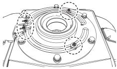
lowing figure. Pass the de-icer power cable through locking wire saddles (1) to (6).
