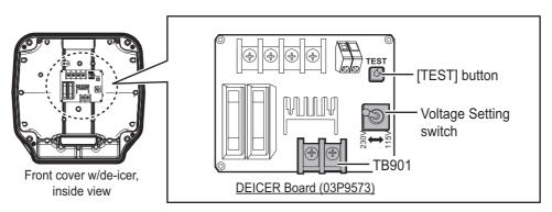
Remove four bolts then spread open the right and left heater elements on the front cover.
