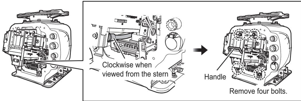
4. Remove the RF unit with the handle.
