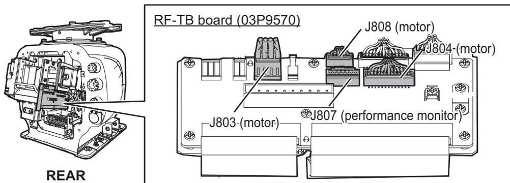
3. Disconnect the coaxial cable and unfasten four bolts to enable removal of the RF unit.
