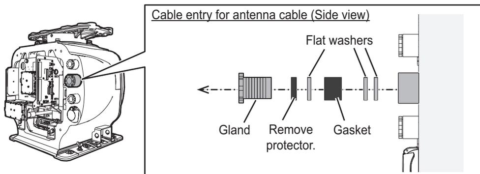
6. Slide the cable gland, the gasket and three flat washers onto the cable.
