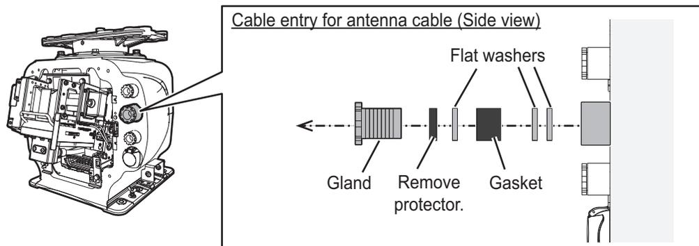
6. Slide the cable gland, the gasket and three flat washers onto the cable.
