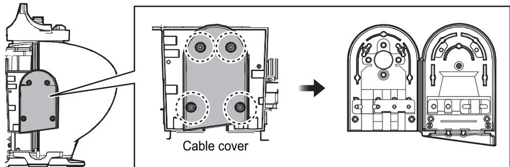
**Note:** The orientation of the cable entrance can be changed. See "How to change the orientation" on page 2-10.
