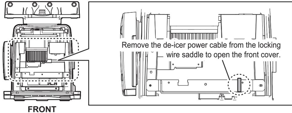
**Note 2:** For the de-icer, take care not to hit the heater elements on the chassis or radiator. If the heater hits something, unfasten the fixing screws for the heater to adjust the position of the heater. Then fix the heater again.
