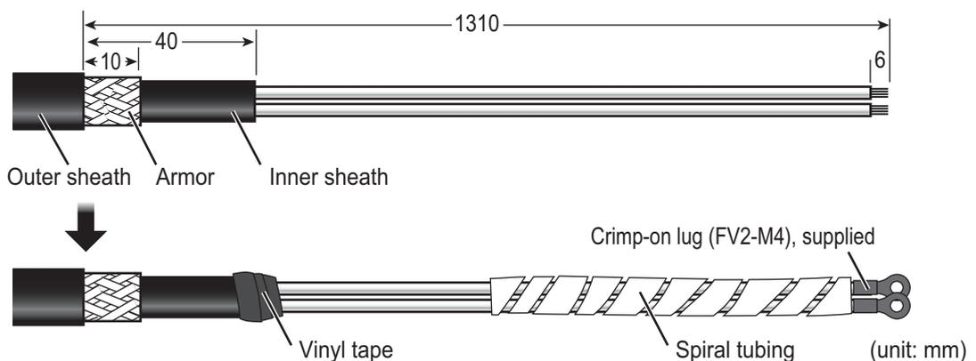
**2.4.2 How to connect the cables for S-band (TR-UP, magnetron) radar**
