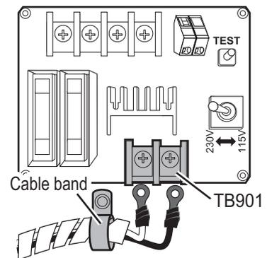
\*: For the DE-ICER installation kit, unfasten the cable band on the supplied cover. (The original cover can be discarded.)
