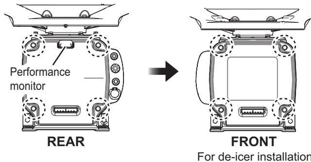
**Note:** The cable for the performance monitor is connected between the rear cover and the RF-TB Board in the antenna unit. Open the cover slowly to prevent damage to the cable and connector.
