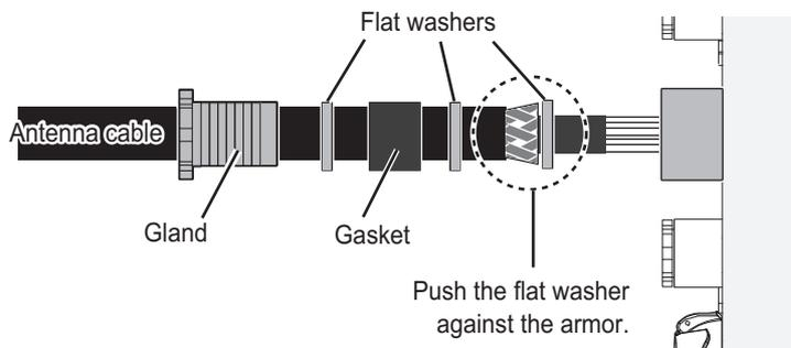
9. Pass the antenna cable through the cable entrance.
