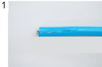
1 Expose inner vinyl sheath.
