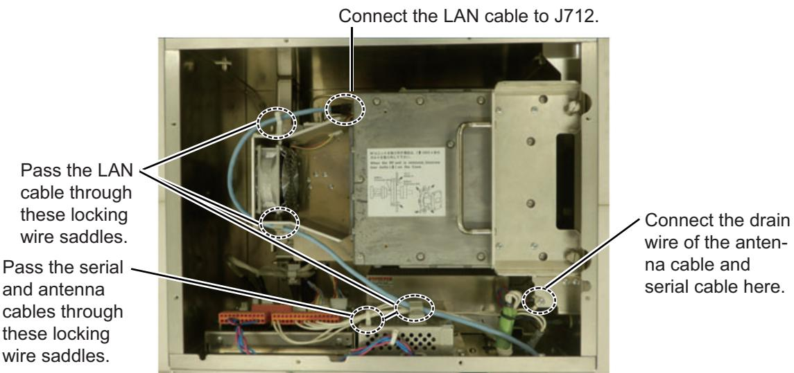
5. Check that cables are lying in their cable slots then fasten the cable clamp.
