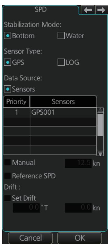
[Stabilization Mode]: Select the water stabilization mode: Select [Bottom] for ground stabilization, or select [Water] for sea stabilization.
