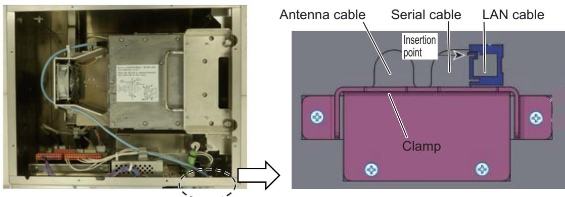
3. Connect the power line of the serial cable to the RF-TB Board as shown in the figure below.
