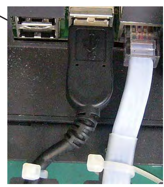
Fix USB cable to the metal fixture with binding ties.
