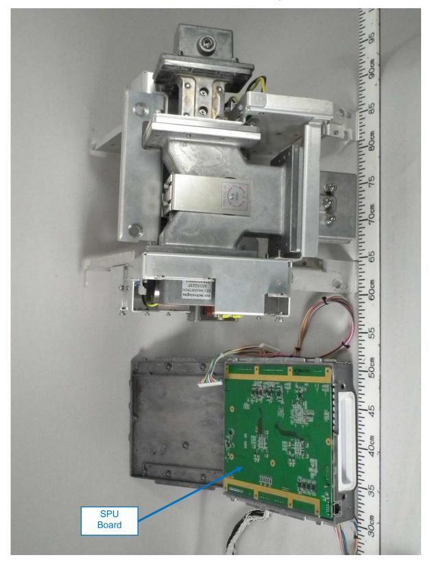
1.1.8 Back of Bottom block (with base plate opened, showing SPU Board 03P9561)
