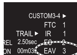
“EAV” (Echo average) icon (at the bottom right corner on the screen)
