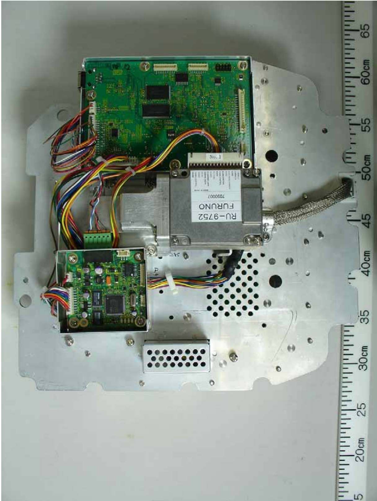
Fig. 1.1.10 Transceiver module Bottom View (with Shield-covers removed, showing NMEA2000 Board 03P9462 (left), RXM module RU-9752 (center) and SPU Board 03P9455 (right))
