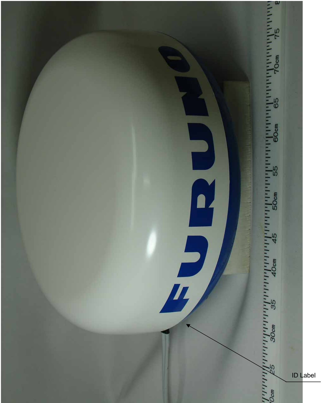
ID Label is affixed on the Radome base.
