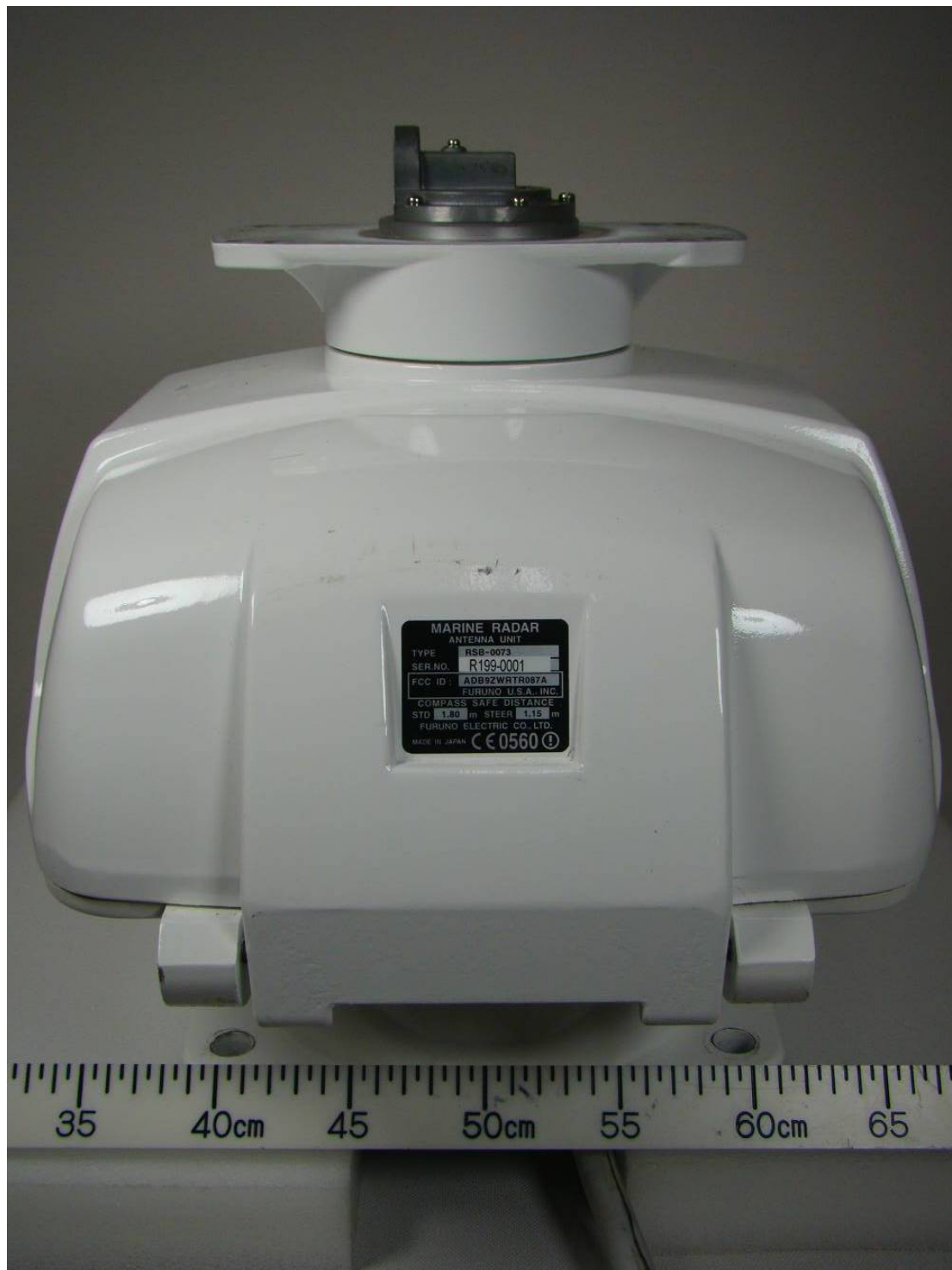
ID Label is affixed on the Scanner Case of the Antenna unit.
