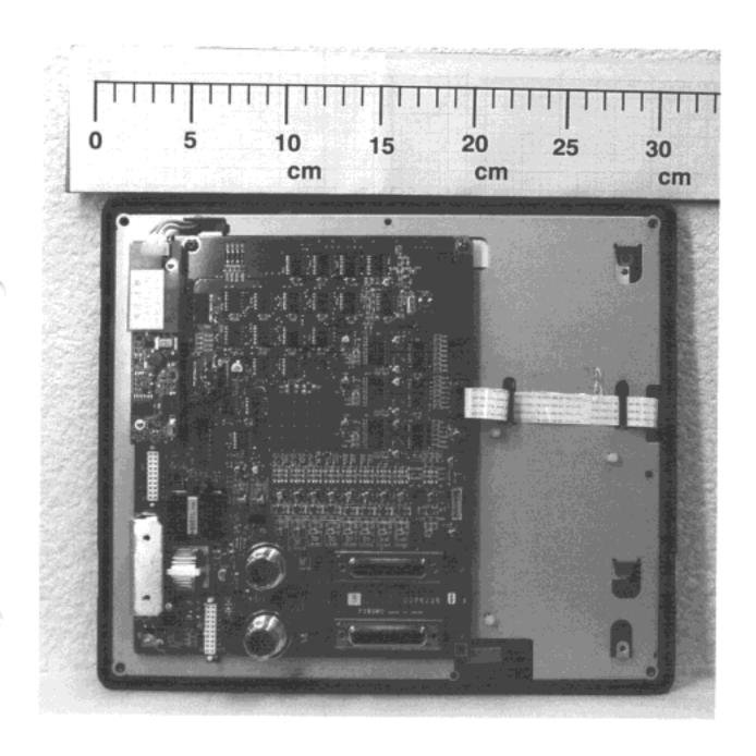
Photo 10.3 LCD Monitor Unit Inside View (cover removed) (showing MCU board (02P6225))
