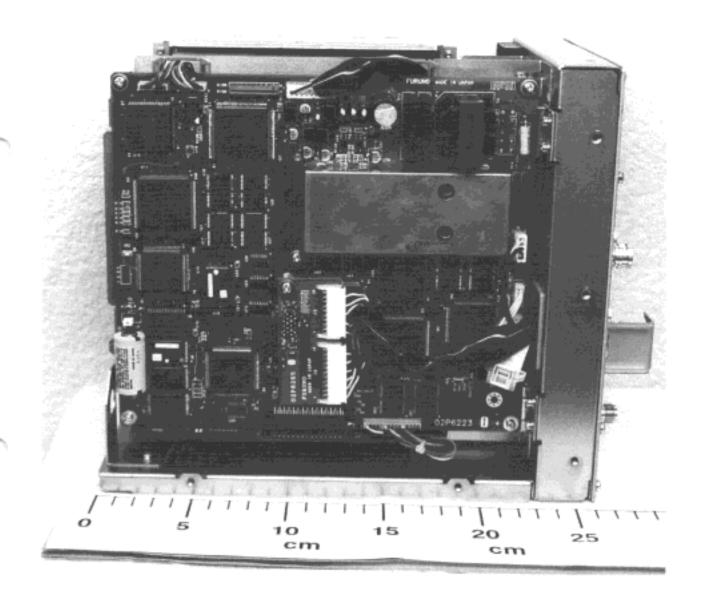
Photo 10.6 Processor Unit Right Side View (cover removed) (showing PSP board (02P6223))
