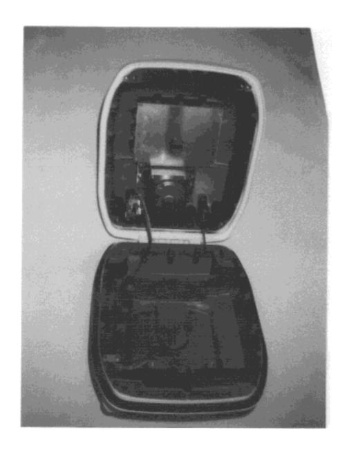
Photo 10.11 Radar Antenna Unit (RSB-0082) Inside View (cover removed)
