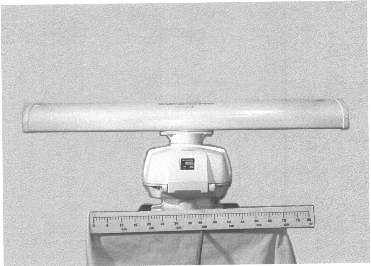
Photo 10.10 Radar Antenna Unit Rear View
