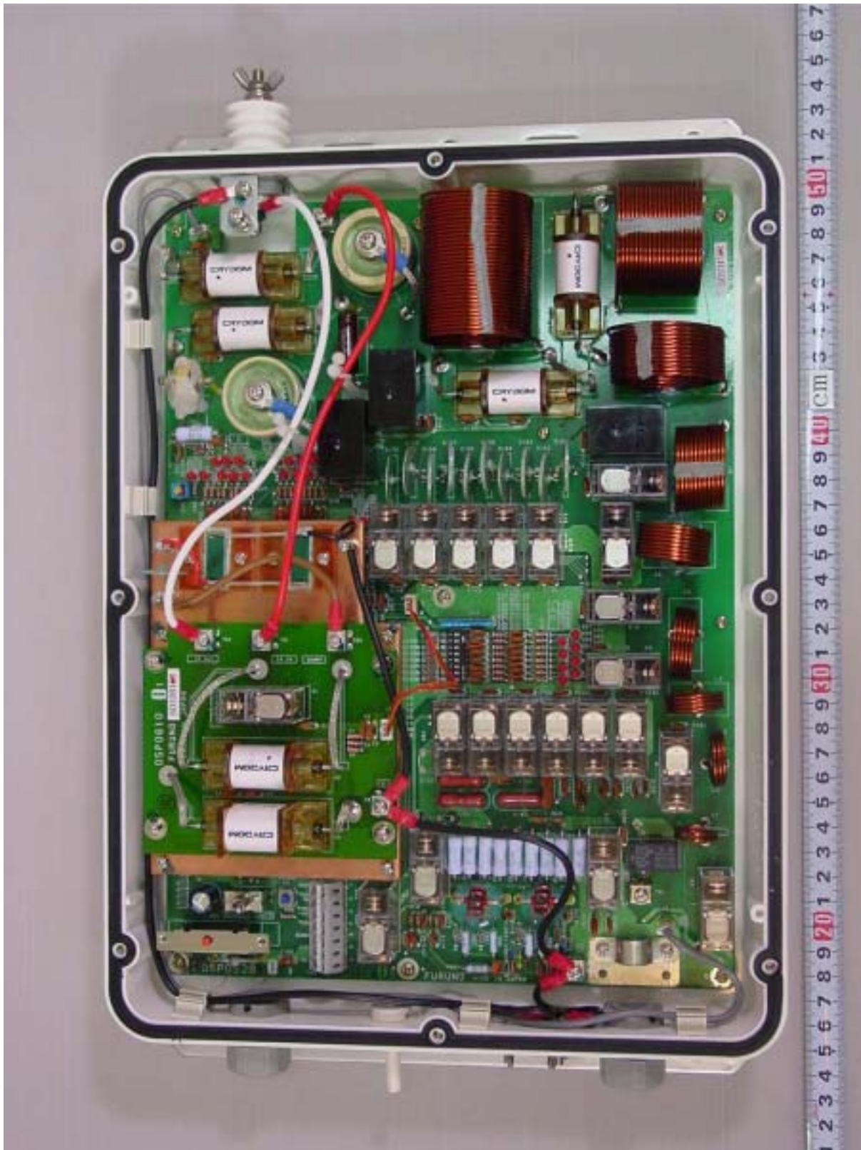
B.2 Inside View (showing COUP Board 05P0528 with DUMMY LOAD Board 05P0610 mounted)
