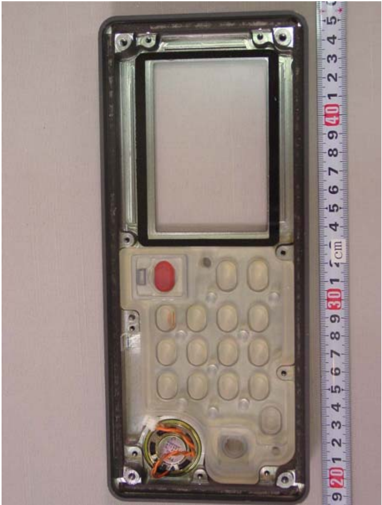
C.7 Inside View (with PANEL Board removed, showing Back of Front Panel)
