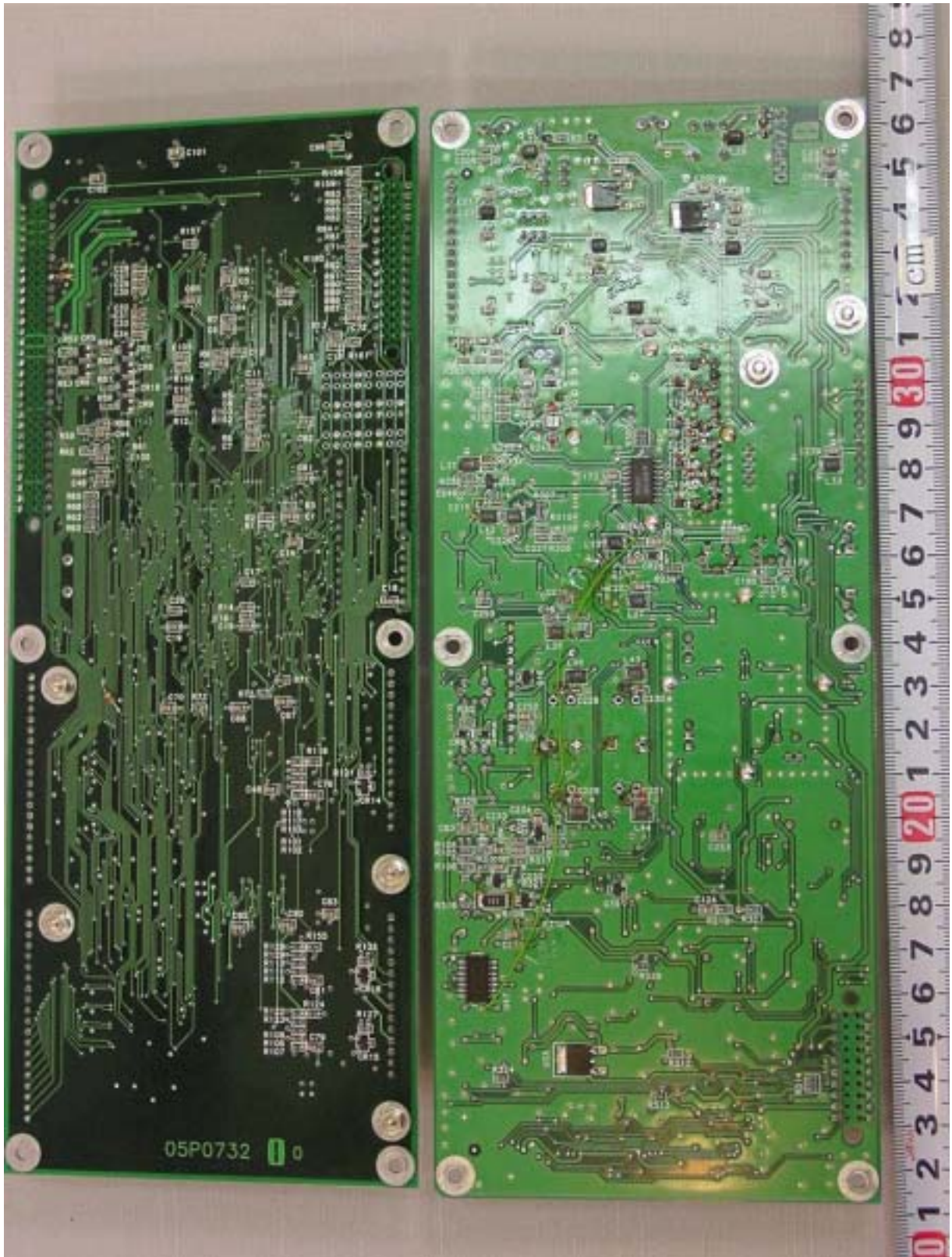
A.10 T-CPU Board 05P0732 (left) and TX-RX Board 05P0733 (right) Rear side
