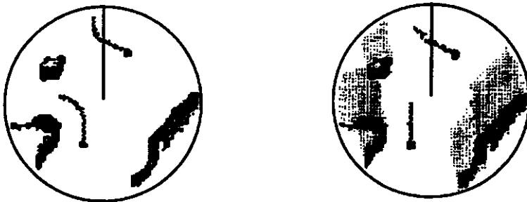
(a) True target trails - no smearing of stationary targets (b) Relative target trails - all targets moving relative to own ship
