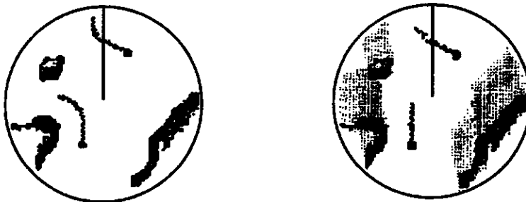
(b) Relative target trails - all targets moving relative to own ship
