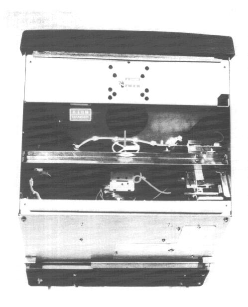
Display Unit Top View (cover removed)
