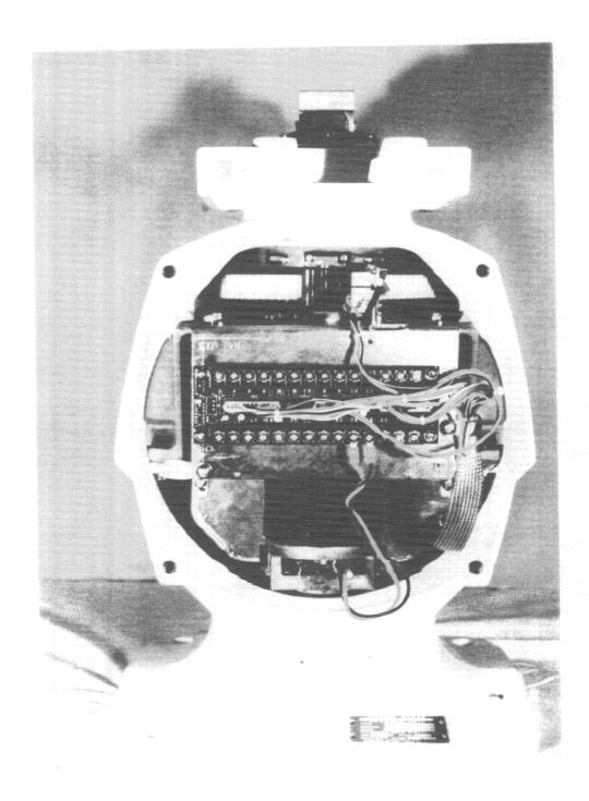
Scanner Unit Inside View (showing TB board (03P9242))
