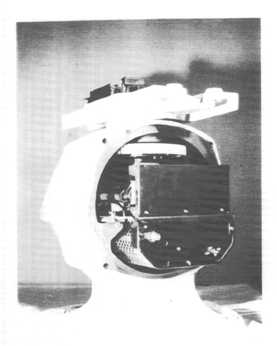
Scanner Unit Inside View (Cover Removed)
