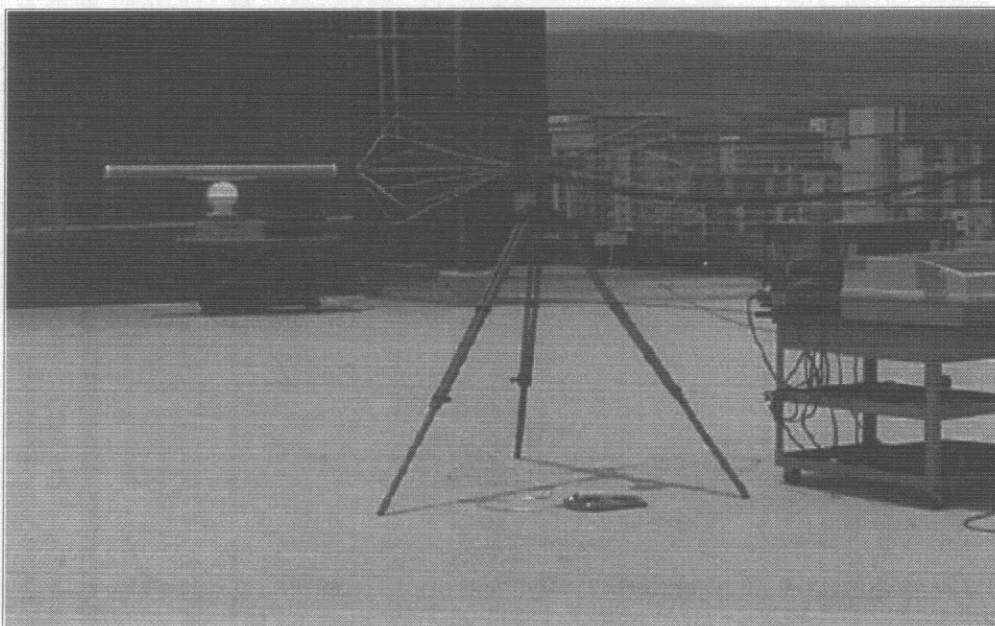
Fig. 7.2 Measuring Antenna: Biconical Antenna Model BIA-25 of Electro Metrics Frequency Range: 20 MHz - 200 MHz
