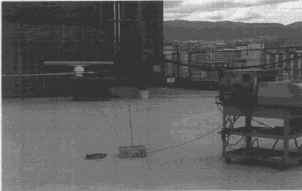
Fig. 7.1 Measuring Antenna: Broadband Rod Antenna Model 95010-1 of Advanced Electronics Frequency Range: 10 kHz - 20 MHz
