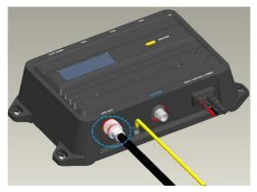
Step 3 Tighten the antenna hand tight.
