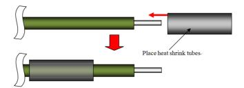
Step 3 Move the heat shrink tubes to the soldered connection, and then apply heat to the tubes.
