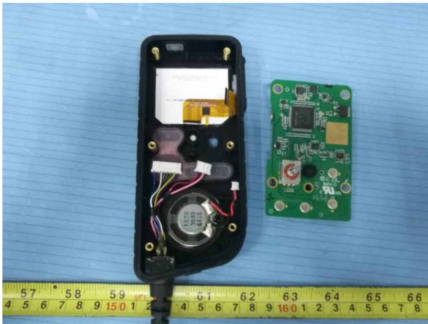
EUT (Handset) – Cover off View 2
