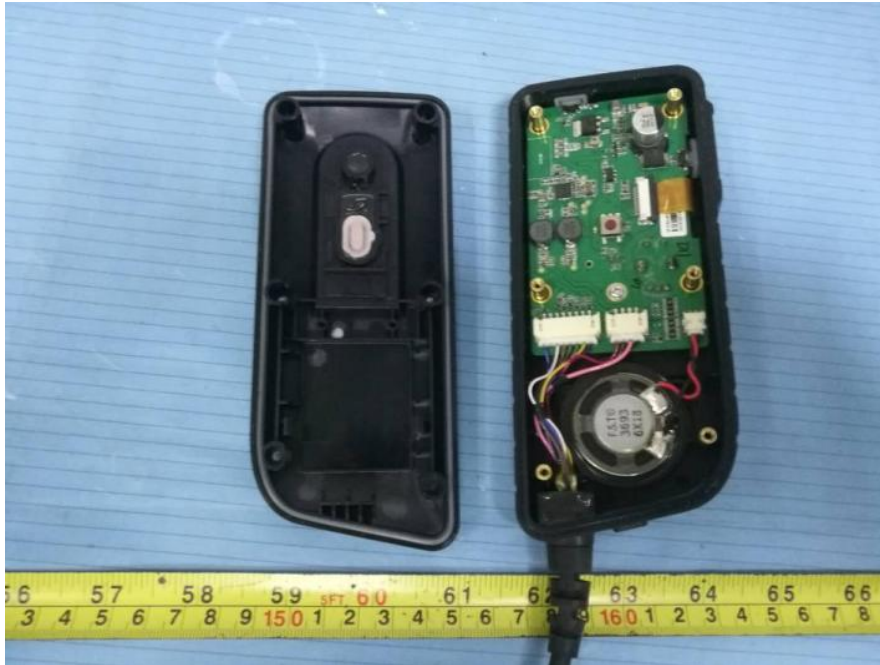
EUT (Handset) – Cover off View 1
