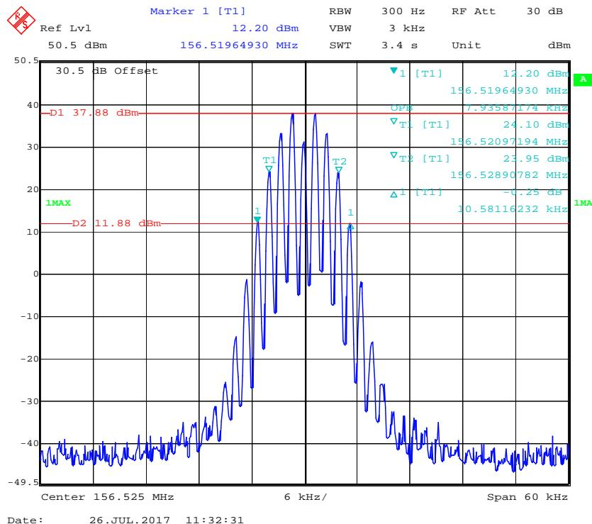
**99% Occupied Bandwidth & 26 dB Emissions Bandwidth (156.525 MHz, DSC1300, Low Power)**
