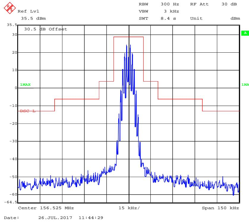
**Emission Mask, (DSC2100Hz, High Power)**
