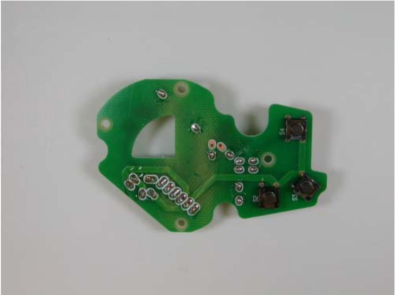
Microphone PCB - rear view
