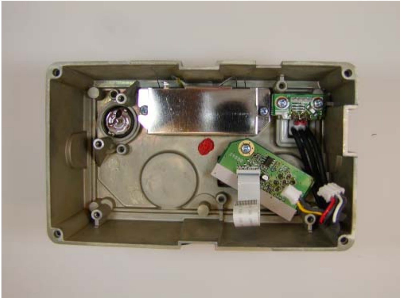
Rear chassis with main PCB removed
