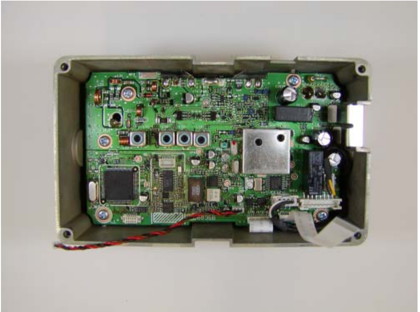
Rear chassis showing main PCB
