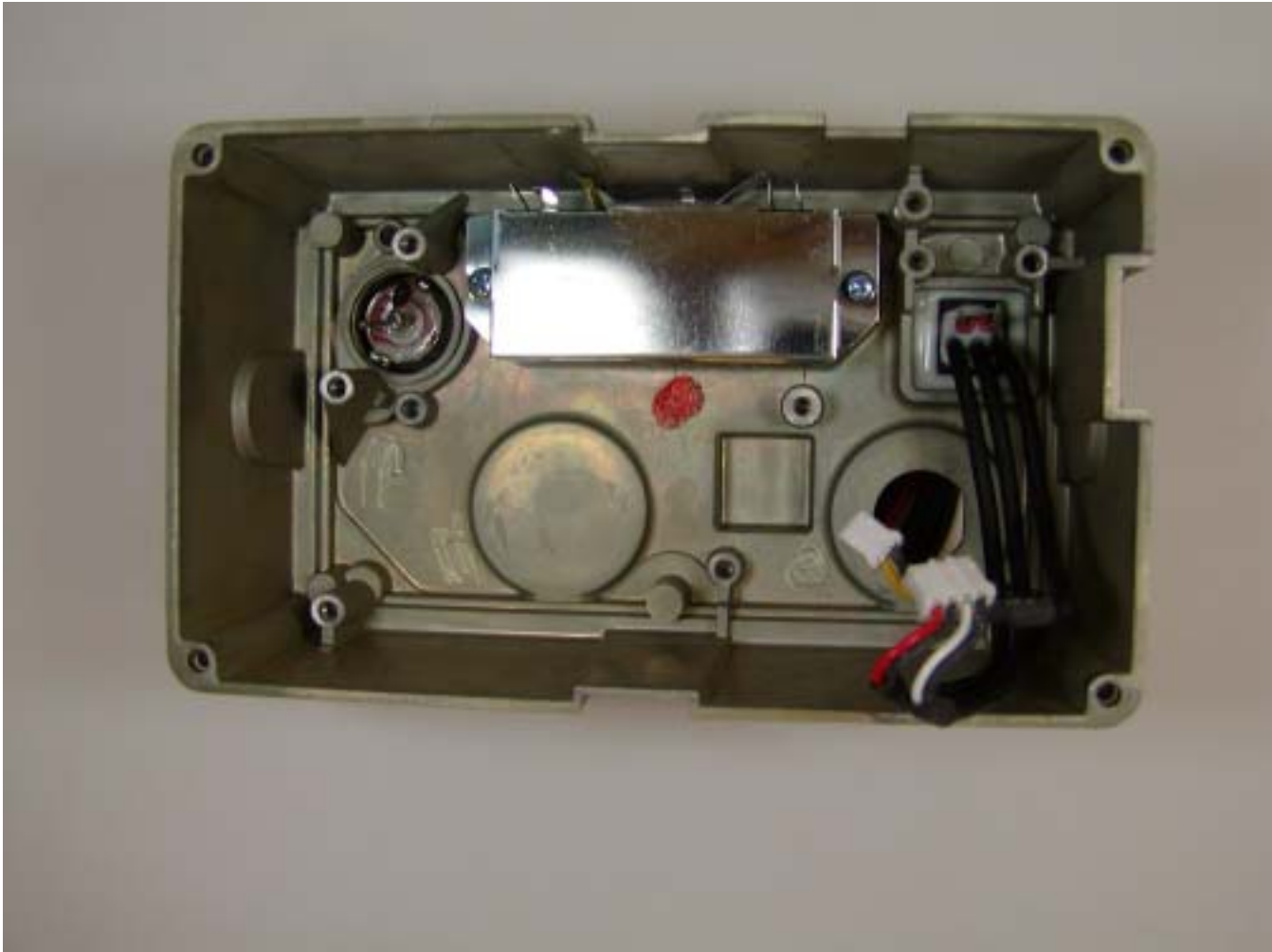
Rear chassis removing all PCBs
