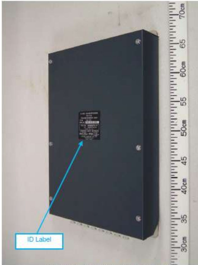
ID Label is affixed on the top of Transponder unit, FA-1701.
