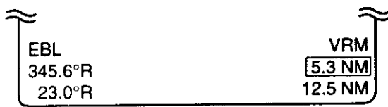
Figure 2-8 Display bottom, showing location of EBL and VRM readouts
