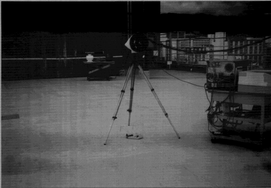
Fig. 7.3 Measuring Antenna: Conical Log-Spiral Antenna Model LCA-25 of Electro Metrics Frequency Range: 200 MHz - 1 GHz Result: Graphs 7.1 to 7.5
