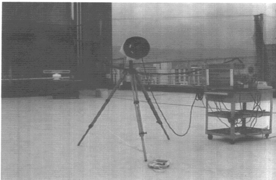
Fig. 7.3 Measuring Antenna: Conical Log-Spiral Antenna Model LCA-25 of Electro Metrics Frequency Range: 200 MHz - 1 GHz
