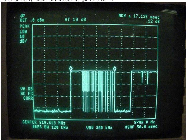
The plot was captured using a continuous trigger with max hold, pressing view when the pulse was captured. Please disregard the partial pulse on the right of the display.
