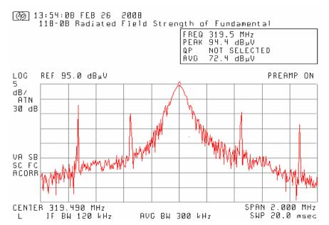
Note: The transients shown on each side of the transmitting frequency are occasional and have no significant quasi-peak or average values.
