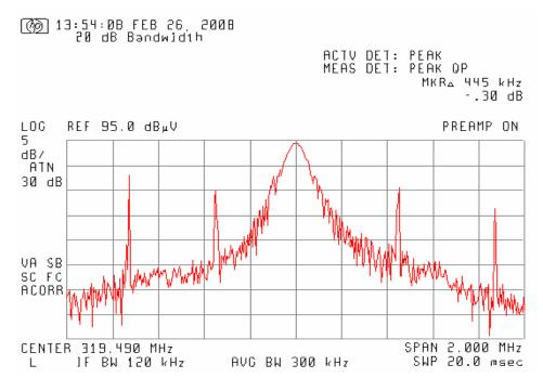
Note: The transients shown on each side of the transmitting frequency are occasional and have no significant quasi-peak or average values.
