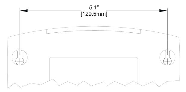
The illustration is drawn at a one-to-one scale, which means that when printed, it provides the exact dimensions required to mount the unit.
