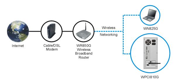
In the example above, the Internet communicates with the modem which communicates with the router. The router acts as the gateway to your network, sending information to whichever device asks for information. The PCI adapter card enables your desktop computer to be part of the wireless network.
