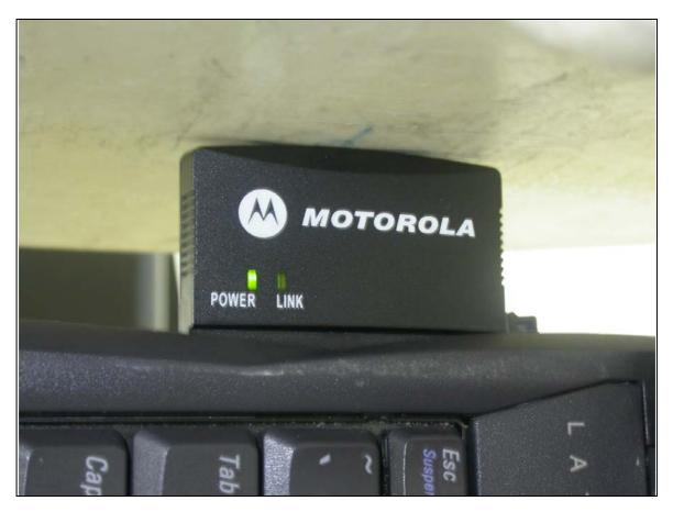
The tip of the EUT to the phantom distance is 0mm
