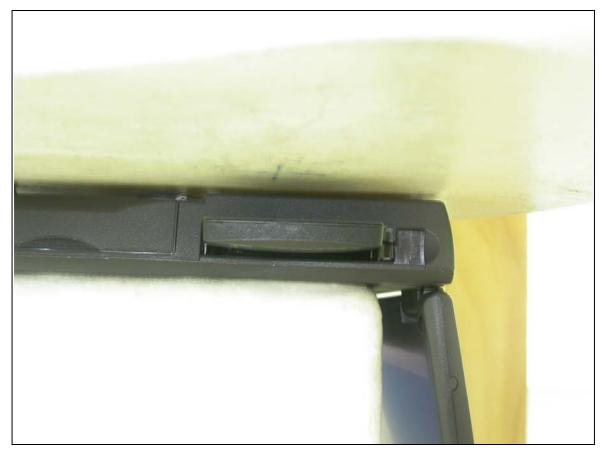
The bottom of the EUT to the phantom distance is 15mm
