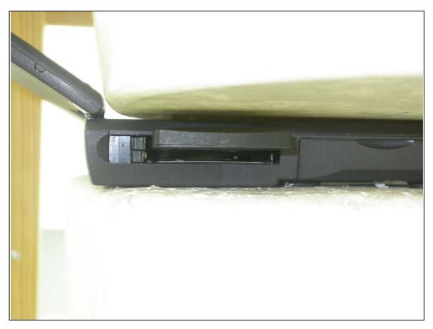
The front of the EUT to the phantom distance is 7mm
