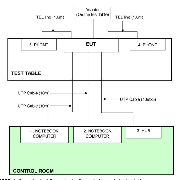
**NOTE:** 1. Support units 1-3 were kept in the control room during the test.
