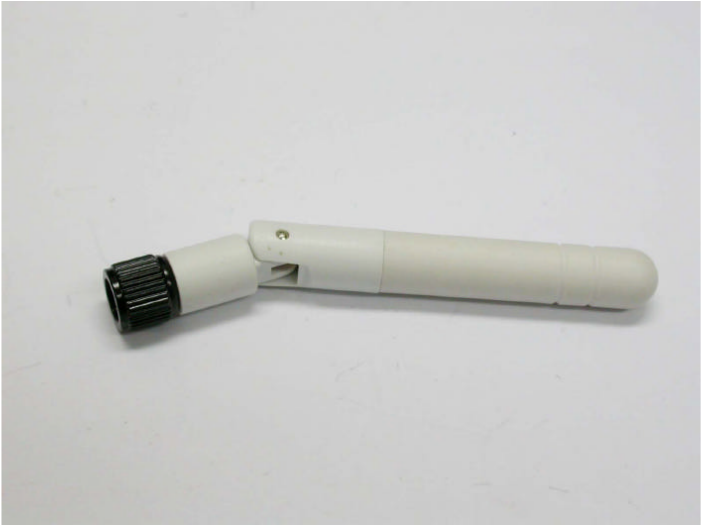
Antenna type 1: Reverse SMA connector, dipole antenna
