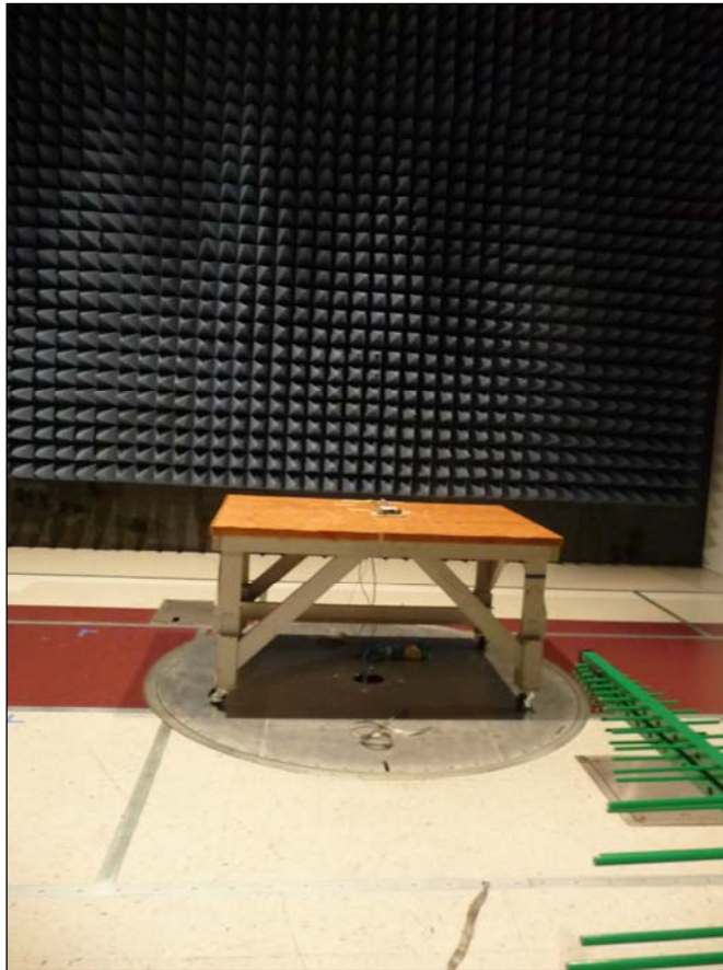
Photograph 2. Radiated Emissions Test Setup, Antenna
