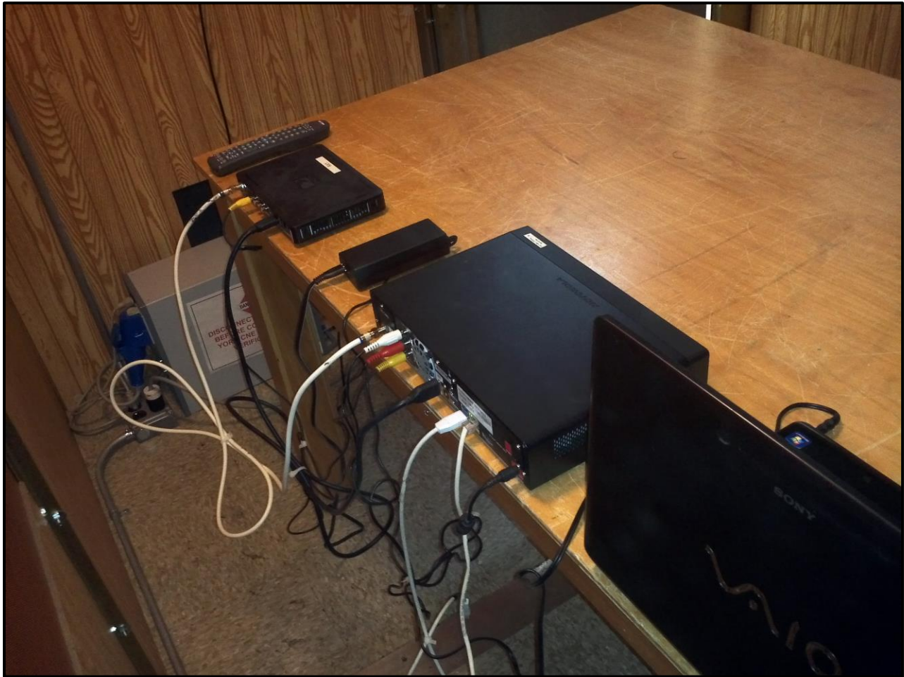
Photograph 6: Conducted Emissions Testing – Back View
