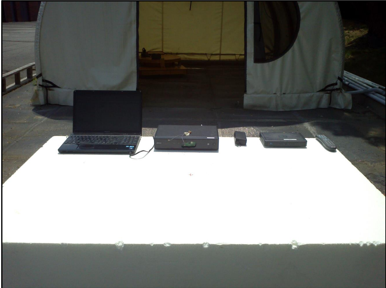
Photograph 3: Radiated Emissions Testing – Front View
