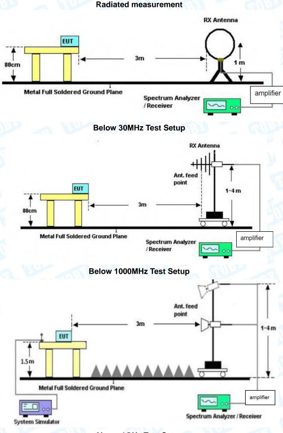
Above 1GHz Test Setup
