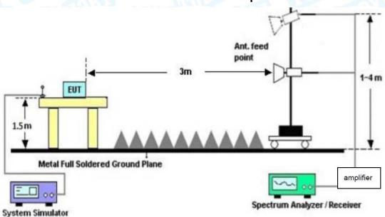
**Above 1GHz Test Setup**
