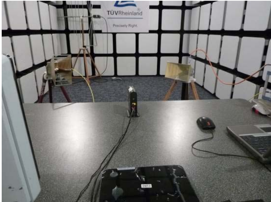
Figure 27: Dynamic Frequency Selection Test Setup – Rear View
