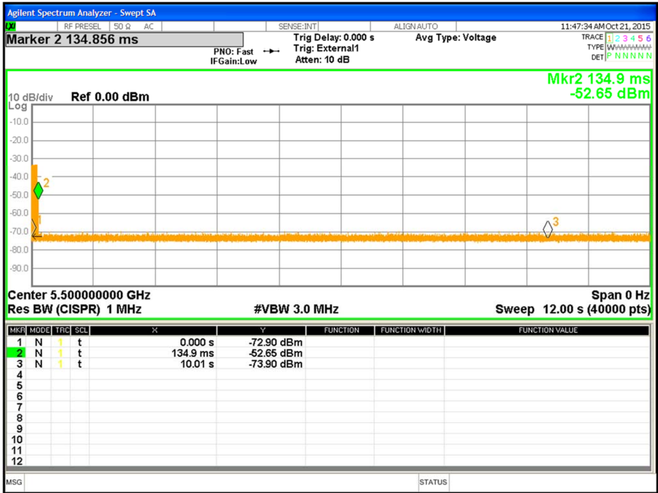
Figure 15: Channel moving time at 5500MHz Plot _with 40MHz BW
