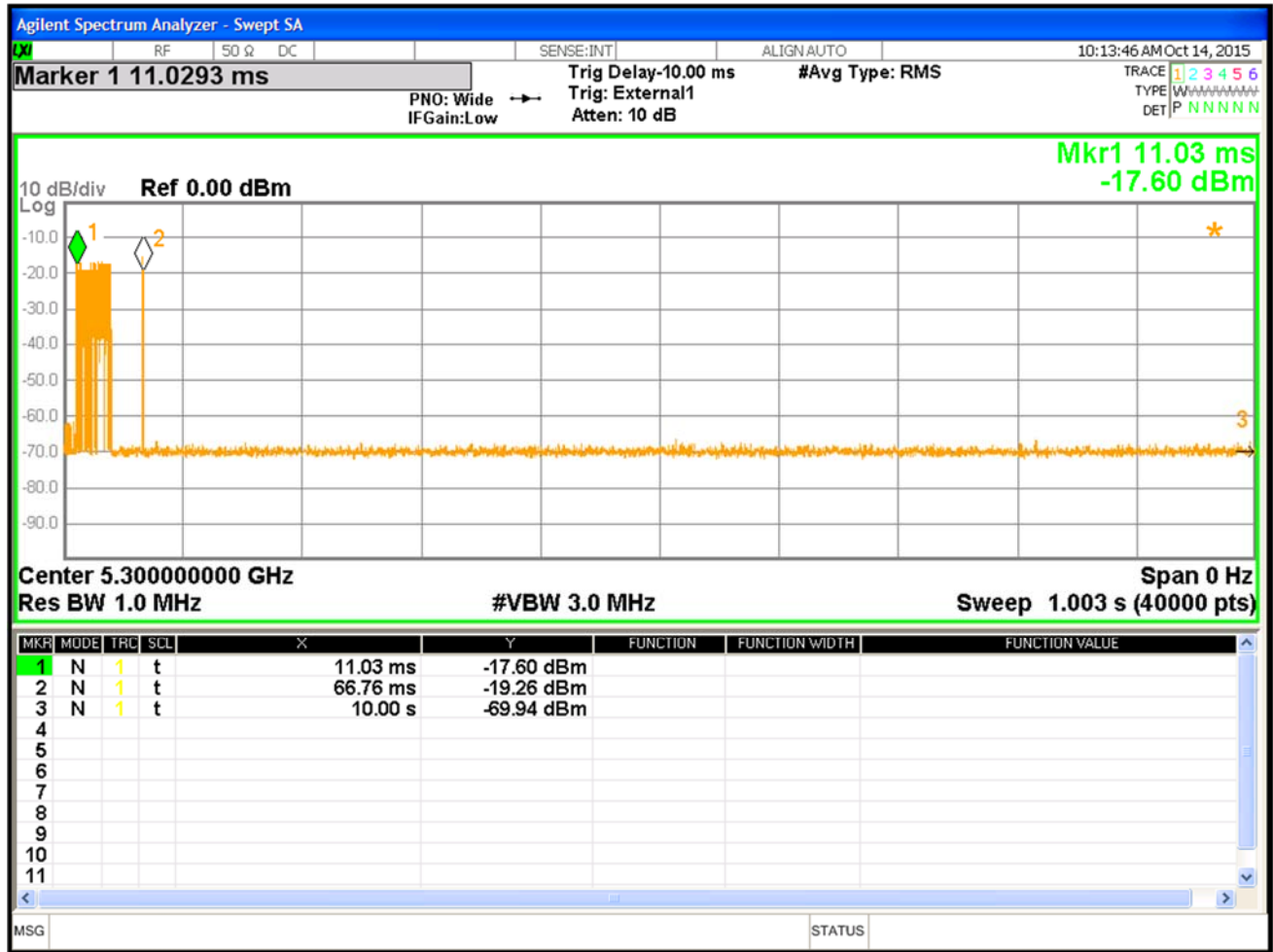
Figure 7: Channel moving time at 5300MHz Zoom in Plot with 40MHz BW
