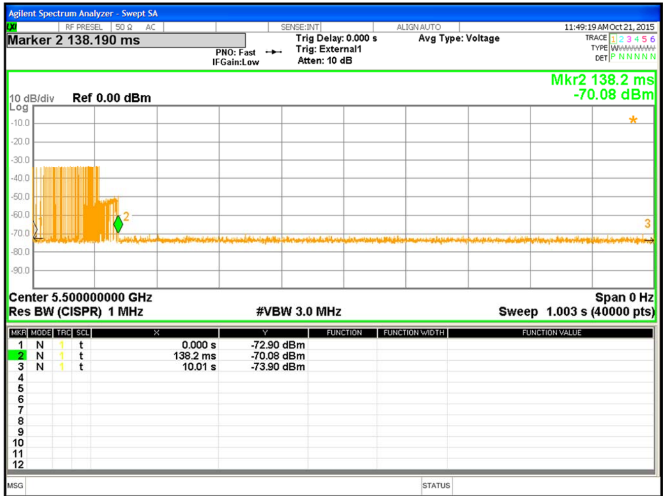
Figure 16: Channel moving time at 5500MHz Zoom in Plot _with 40MHz BW
