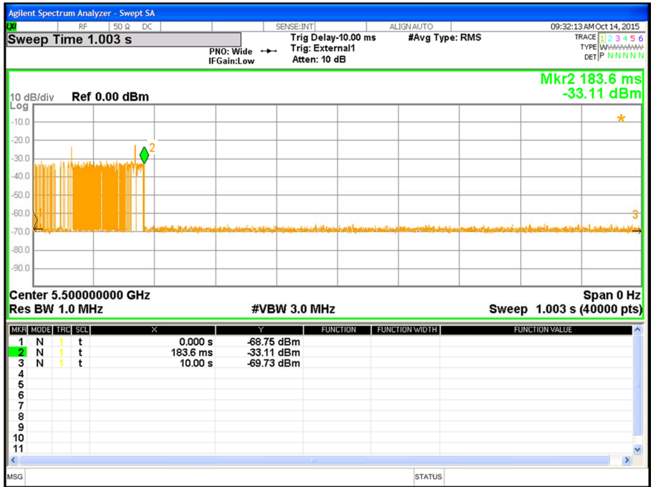
Figure 13: Channel moving time at 5500MHz Zoom in Plot _with 20MHz BW
