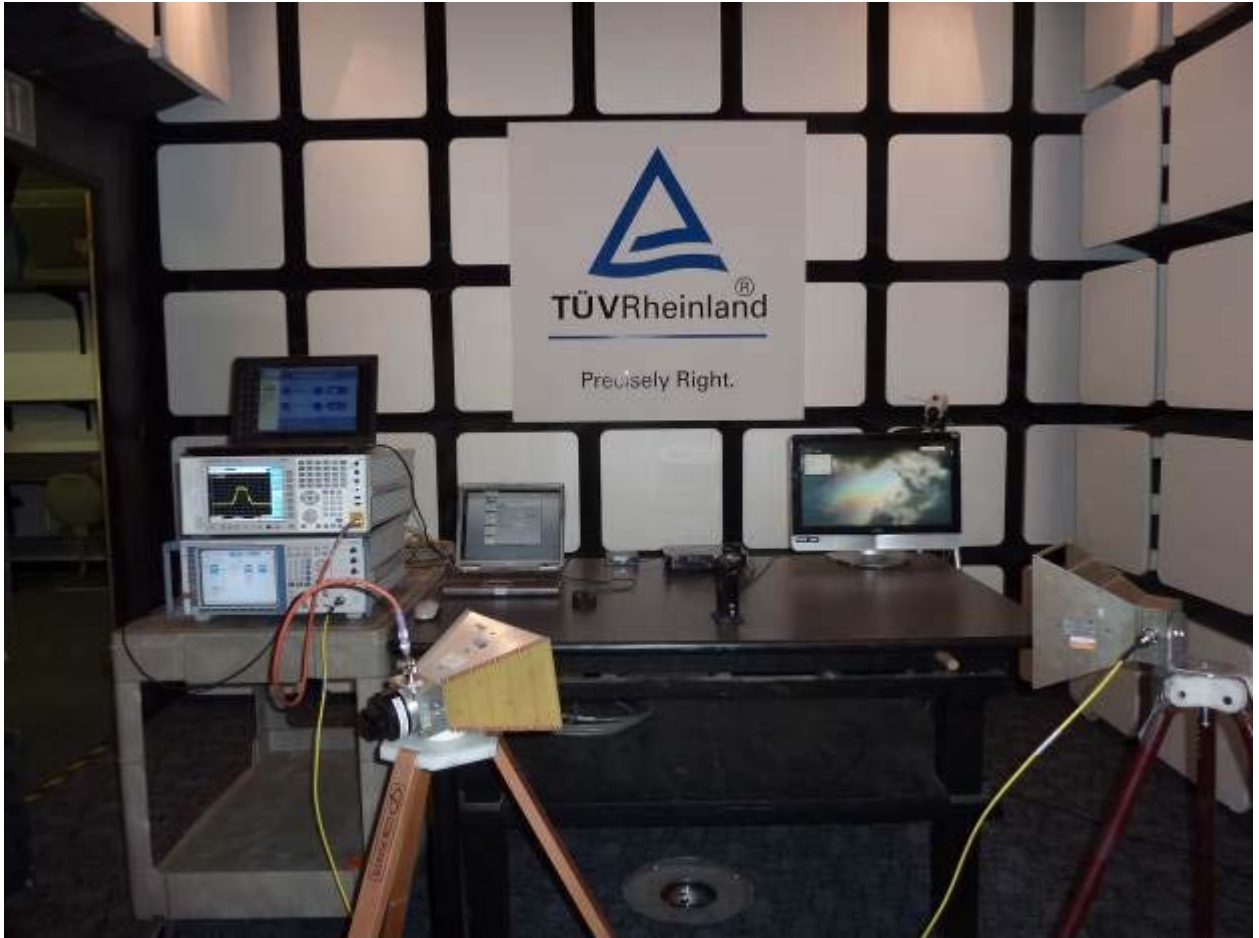
Figure 26: Dynamic Frequency Selection Test Setup – Front View
