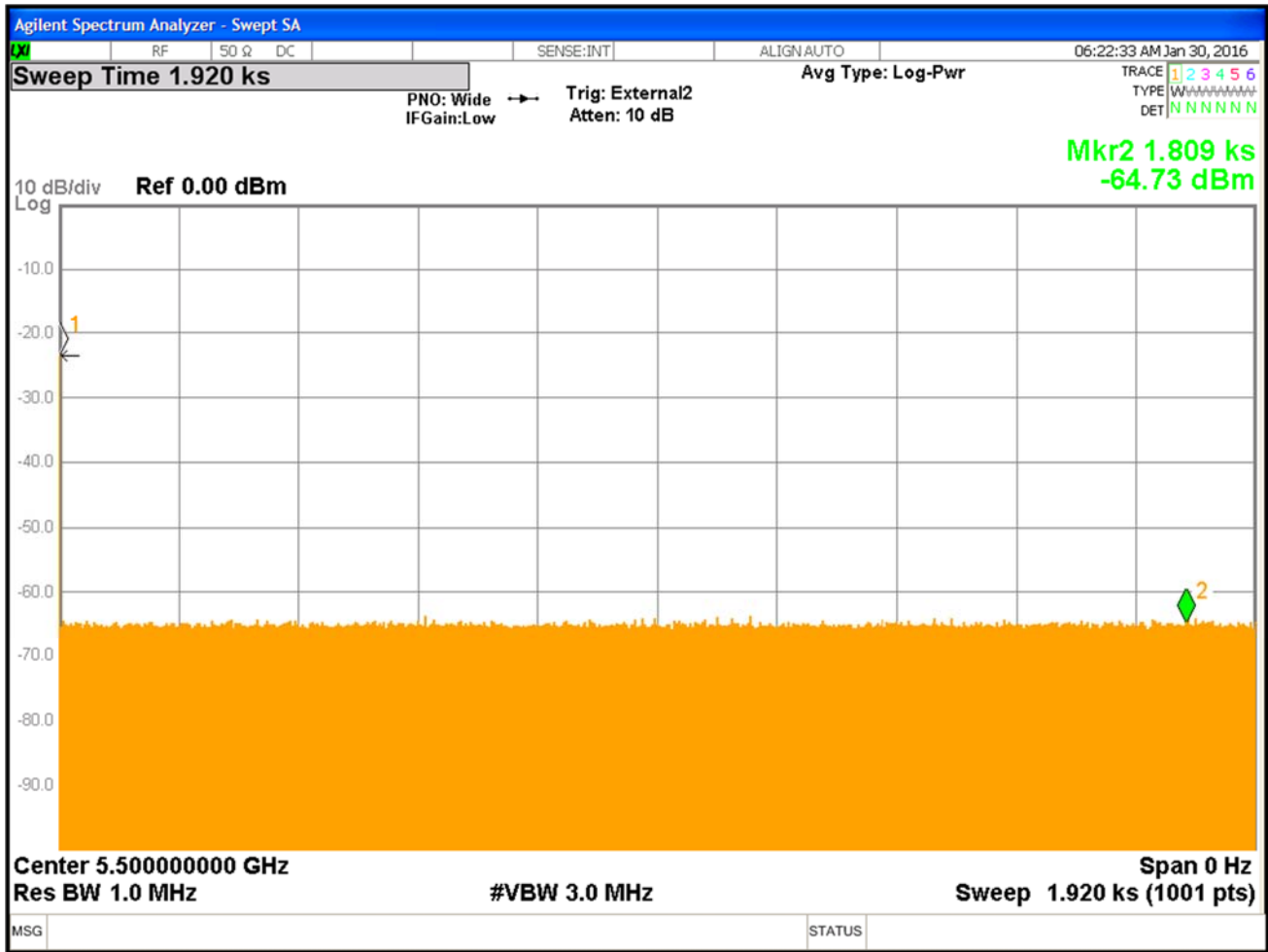
Figure 14: Channel Non-occupancy plot for 32min at 5500MHz with 20MHz BW Master and slave moved to Ch#161
