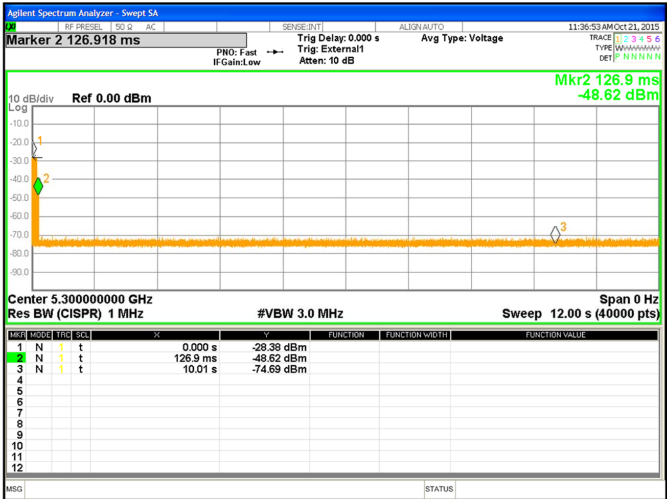
Figure 3: Channel move time, signal plot for 12Secs at 5300 MHz for 20MHz BW
