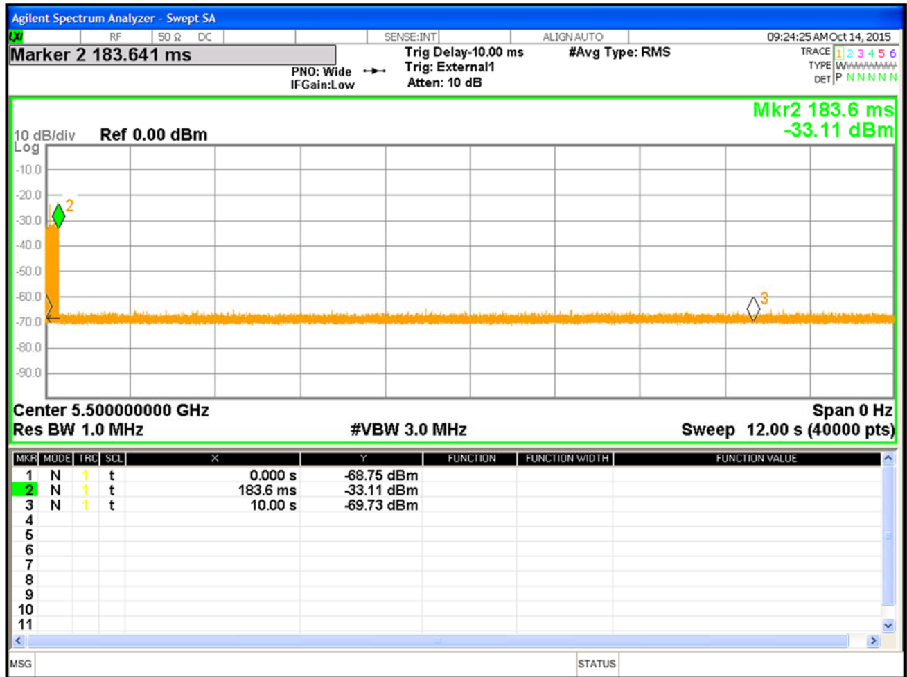
Figure 12: Channel moving time at 5500MHz in Plot _with 20MHz BW
