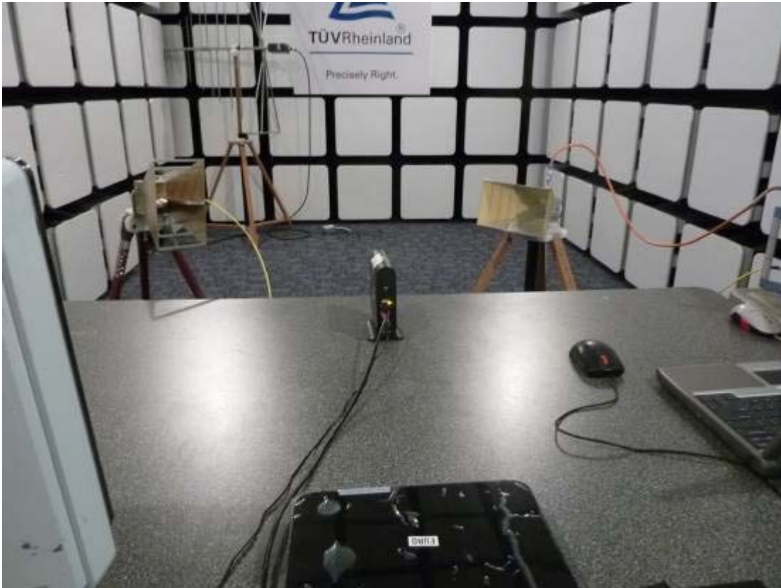
Figure 1: Dynamic Frequency Selection Test Setup – Rear View
