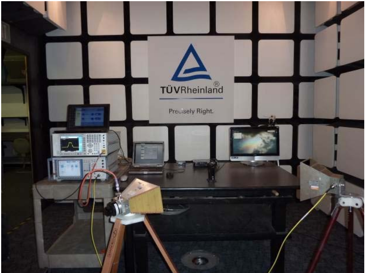
Figure 19: Dynamic Frequency Selection Test Setup – Front View
