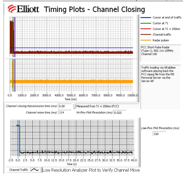
Figure 2 Channel Closing Time and Channel Move Time, n20 mode (VIP2500) - 40 second plot
