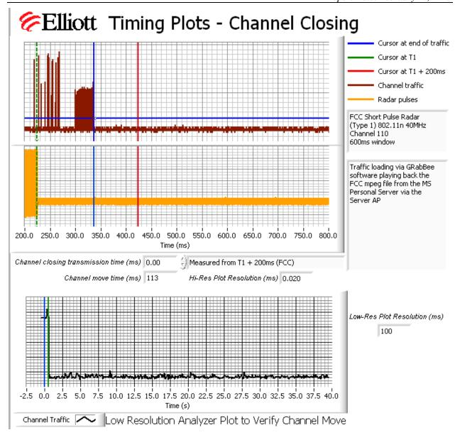
Figure 9 Close-Up of Transmissions Occurring More Than 200ms After The End of Radar (VIP2502)
