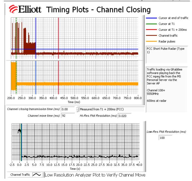
Figure 7 Close-Up of Transmissions Occurring More Than 200ms After The End of Radar (VIP2500)
