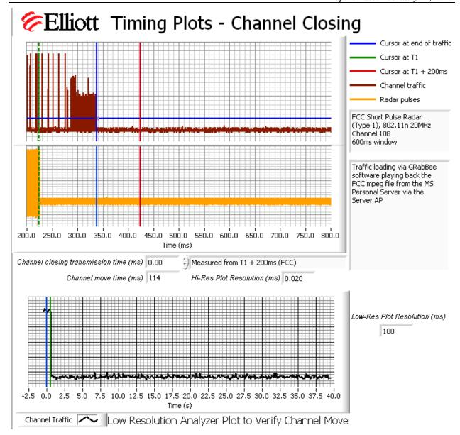
Figure 3 Close-Up of Transmissions Occurring More Than 200ms After The End of Radar (VIP2500)
