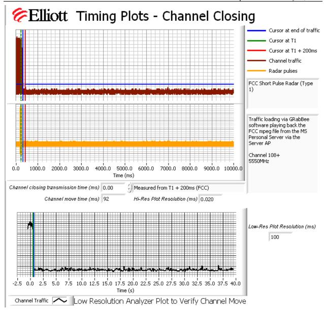
Figure 6 Channel Closing Time and Channel Move Time, n40 mode (VIP2500) - 40 second plot
