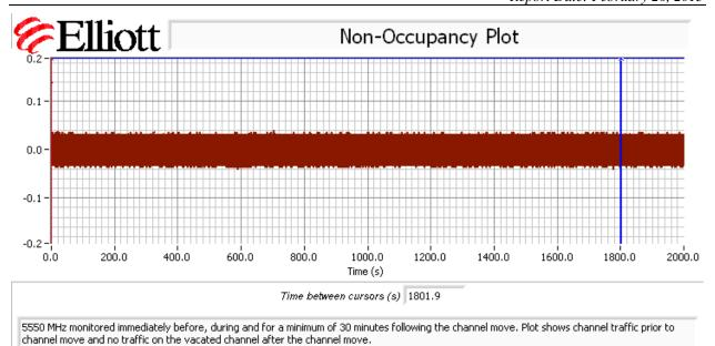
Figure 10 Radar Channel Non-Occupancy Plot (VIP2500)
