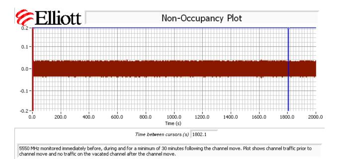
Figure 11 Radar Channel Non-Occupancy Plot (VIP2502)
