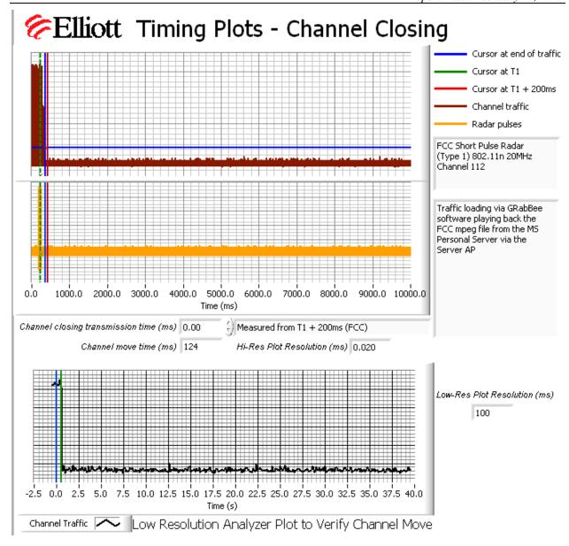
Figure 4 Channel Closing Time and Channel Move Time, n20 mode (VIP2502) - 40 second plot
