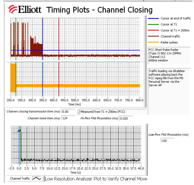
Figure 5 Close-Up of Transmissions Occurring More Than 200ms After The End of Radar (VIP2502)
