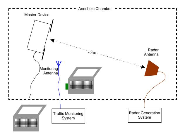
Figure 1 Test Configuration for radiated Measurement Method
