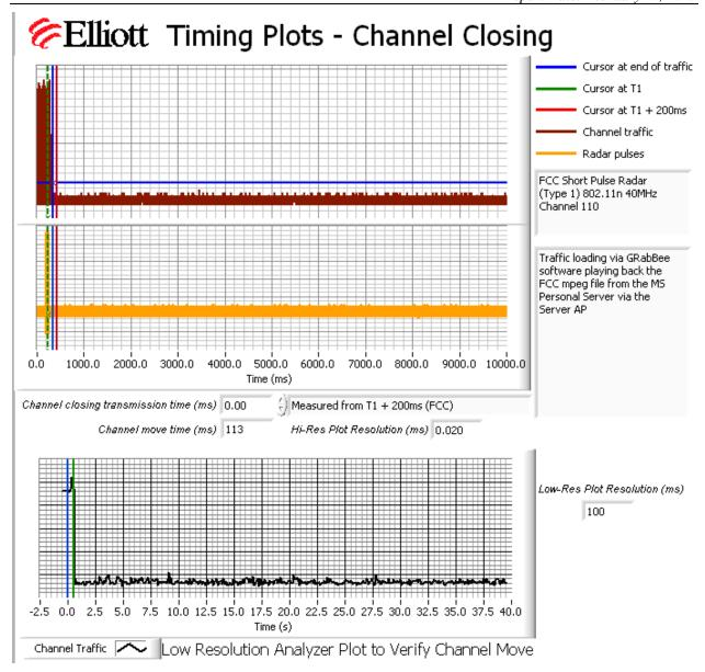
Figure 8 Channel Closing Time and Channel Move Time, n40 mode (VIP2502) – 40 second plot
