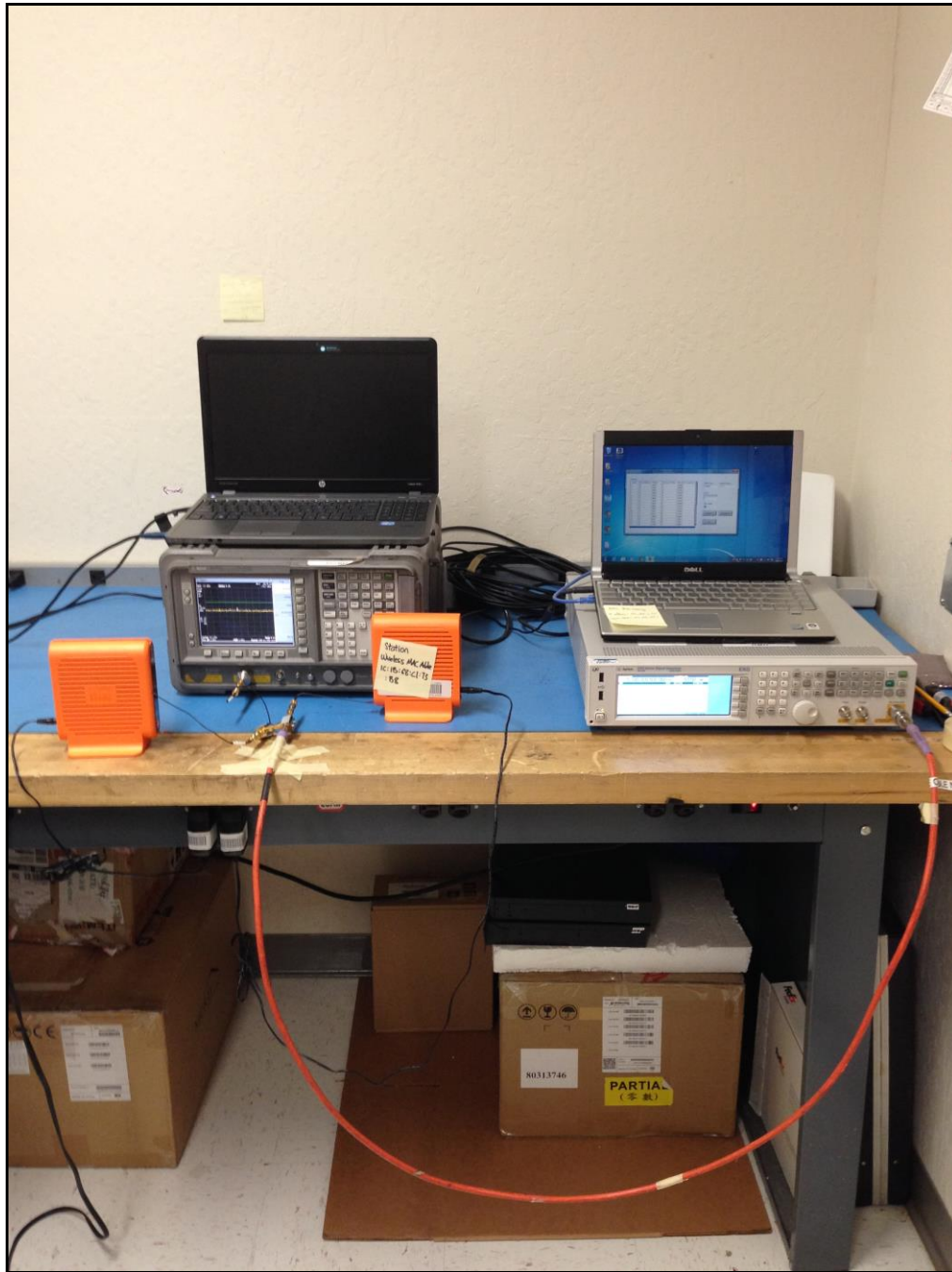
Photograph 2. DFS, Test Setup
