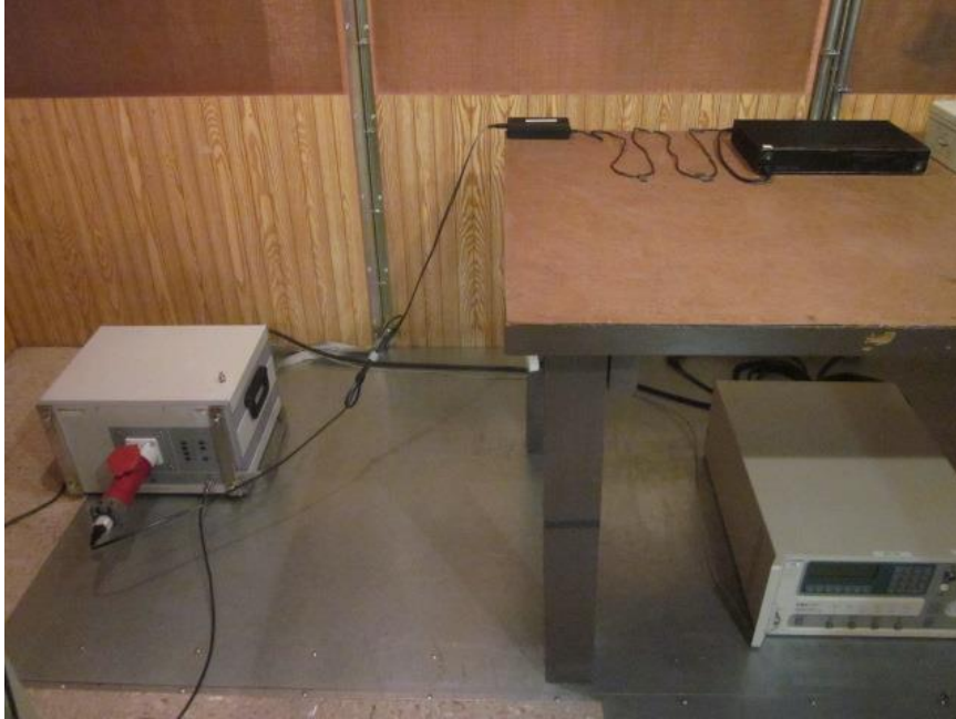
Conducted Emissions Antenna Test Setup Picture
