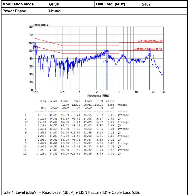
Note 1: Level (dBuV) = Read Level (dBuV) + LISN Factor (dB) + Cable Loss (dB). 2: Over Limit (dB) = Level (dBuV) – Limit Line (dBuV).
